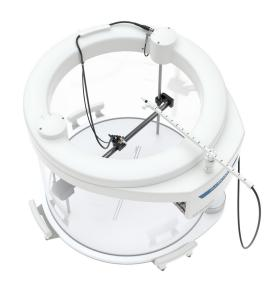
Virtual Reference Detector using Pulse Normalization is an exclusive feature of the SunSCAN 3D that permits accurate scanning without the need of a physical reference detector, simplifying the acquisition of data for small fields.
