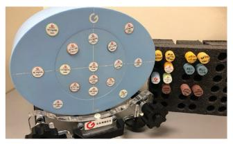
**Figure 1**. The Gammex Multi-Energy CT phantom with tissue-mimicking rods. The picture shows the "body" configuration; the central section of the phantom can be used separatley as a "head" phantom.
